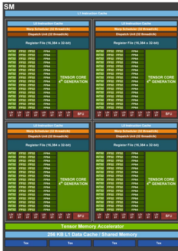
Figure 1 GPUs have blocks of fixed data formats—limiting researchers’ ability to explore new quantization methods. [Source: Nvidia]
